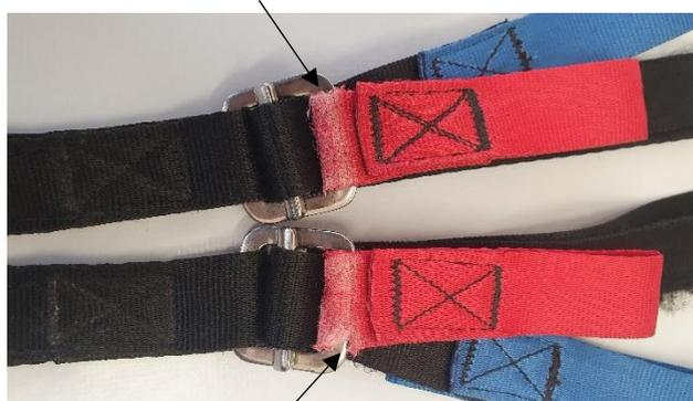
**Significant tear -replace the Backstrap**
